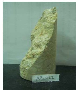
图1 膏溶角砾岩断口的立面图 Fig.1 Elevation drawing of fracture in gypsum breccia
