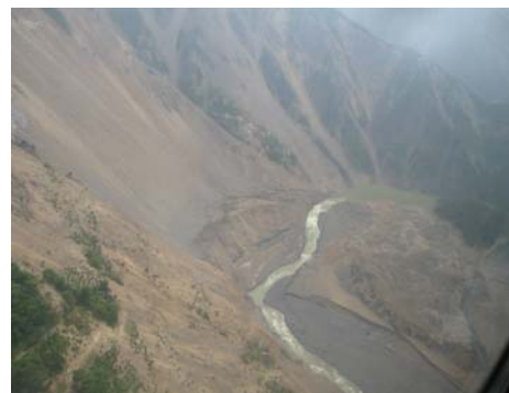
图 4 堰塞坝“6.10”正常泄水后形成的泄流渠(面朝上游) Fig.4 Discharge channel formed after barrier dam overflowing on June 10(facing upstream)
