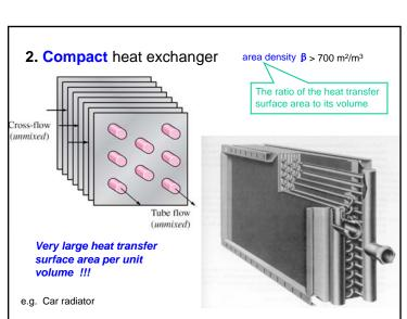
A heat exchanger allows heat to be transferred between two fluids without the fluids contacting each
