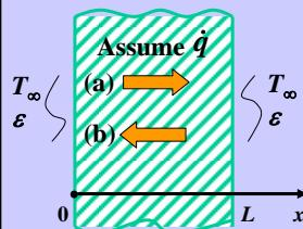
$$-k \left( \frac{\partial T}{\partial n} \right)_s = \varepsilon \sigma (T_s^4 - T_\infty^4)$$
