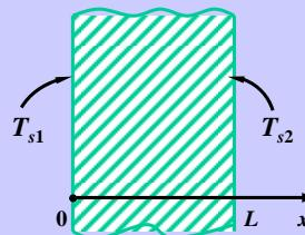
$$T_s = \begin{cases} \text{const} \\ T_{si} \pm Ct \\ \dots \end{cases} \quad (\frac{\partial T_s}{\partial t} = \pm C)$$
