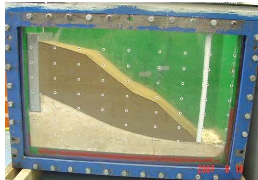
图3 库区滑坡的离心模型图 Fig.3 Picture of centrifugal model for reservoir landslide
