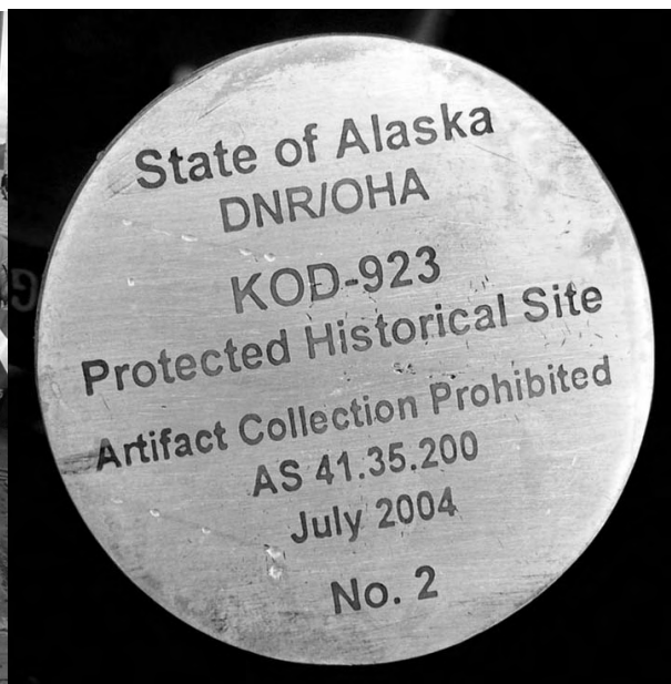
Figure 2. Example of one of the brass survey cap placed on the wreck sites, inscribed with the AHRS site number and proclamation of the site's protected status under State law.
