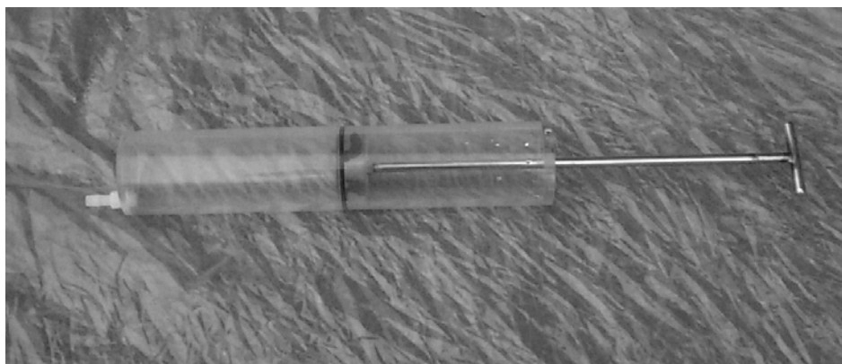
Figure 5. 1L syringe used to sample water from the chambers for Winkler titrations and biogeochemically important chemical constituents.
