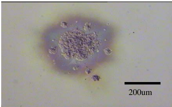
Fig.1 Nomarski optical micrograph of typical damage after 5 shots at 7 \text{ J/cm}^2 for HR coating
