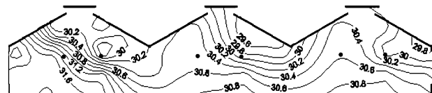
(c) Case 3: nozzle locations of 2.8, 4.7, 10.3, 12.2, 17.8, and 19.7 m from the left wall at the height of 2.7 m with the vertical-upward injection of spray.
