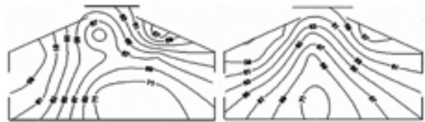
Fig. 3. Comparison of measured (left) and simulated (right) relative humidity in the greenhouse
