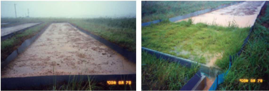
Fig. 4. Flow condition in the field plots during the rainstorm event from August 6 to 8 in 2003 Left: Control plot, Right: 3.0-m-strip plot.
