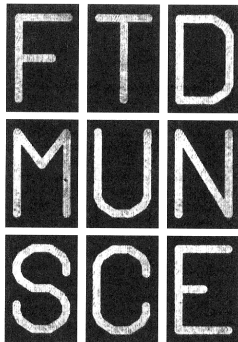
Fig. 6 Nine reconstructions from the batch of 100 holograms using shift multiplexing. Here the spatial separation between successive holograms was 3 \mu\text{m} and L' = 22 mm.
