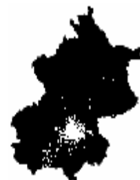
图 9 基于光谱的监督分类和 DEM 提取的北京建成区 Fig. 9 Extracted urban area based on supervised classification and DEM
