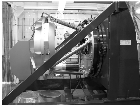
Fig. 2. ELMER Structure and Mechanisms as installed at the IAC Workshop, where the PO team is finishing the integration
