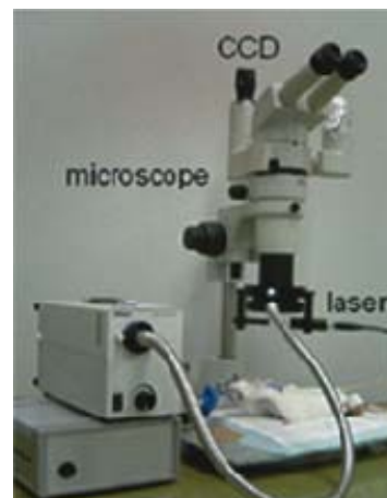
Fig.1 LSF system and experimental setup. Laser light at 780 nm wavelength is reflected by a mirror and irradiates the object.
