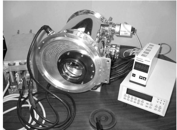
Fig. 1. ELMER CCD camera: LN<sub>2</sub> bath cryostat with CCD head and engineering flat window mounted (middle part), SDSU-II CCD controller (left), and Lakeshore 331 temperature controller and Pfeiffer TPG 261 vacuum gauge controller (right).
