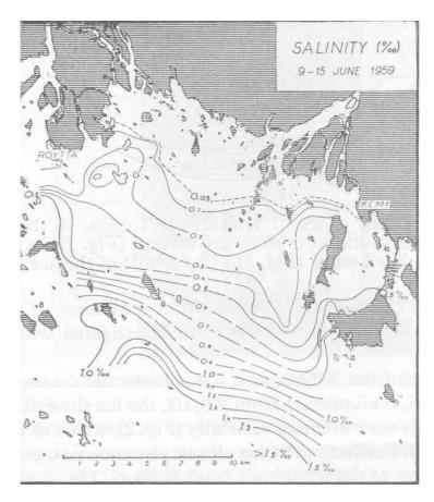
Salinity of the water in the estuary of Tornionjoki river on the northern coast of the Bay of Bothnia. The salinity front in this region was examined for the transition between fresh water ice type and sea ice type (Palosuo, E., 1961. Crystal structure of brackish ice and fresh-water ice. Snow and Ice Commission 54, pp. 9–14, IAHS, Gentbrugge, Belgium). With the permission of International Association of Hydrological Sciences.
