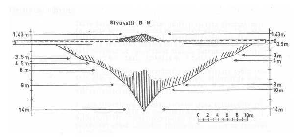
Erkki Palosuo is highly recognised for his extensive investigations of the sea ice ridges in the Baltic Sea. Here a ridge profiled by him in the Bay of Bothnia is shown. The ridges have a key role in the dynamics of sea ice and also in the resistance of drift ice field to ship motion. (Palosuo, E., 1975. Formation and structure of ice ridges in the Baltic. Winter Navigation Research Board, Report 12, Helsinki)
