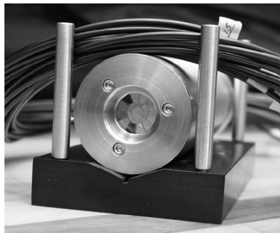
Fig. 2. The completed lens array in its mounting, coupled to the optical fibers.
