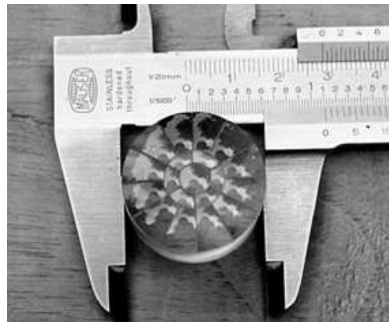
Fig. 1. The lens array. The outer diameter is 28 mm.
