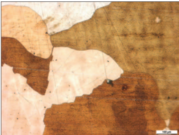
a) as-cast microstructure of 22ct Au without Co
