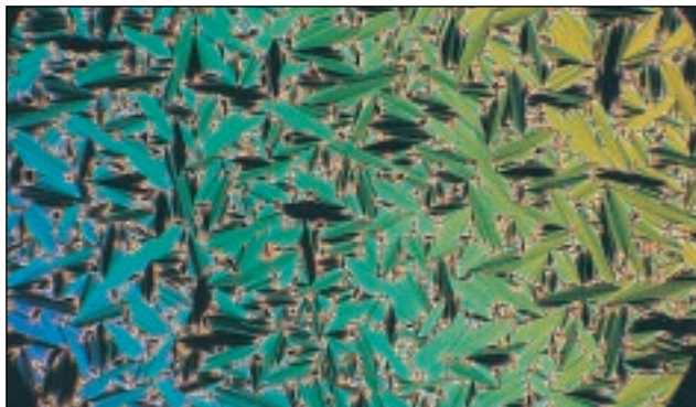
Figure 3 Fan-shaped S_A texture of [ClAu(CNC_6H_4OC_6H_{13})] at 160^\circ C upon cooling from the isotropic state (between crossed polarizers, \times 100 ).
