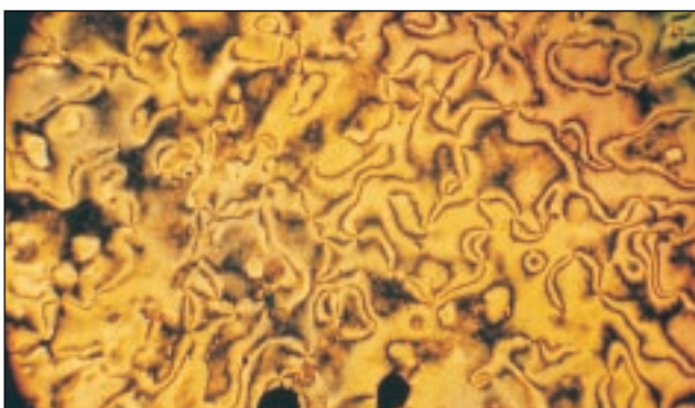
Figure 4 Nematic schlieren texture of [ClAu(CNC_6H_4C_6H_4OC_4H_9)] at 160^\circ C upon heating from the solid state (between crossed polarizers, \times 100 ).
