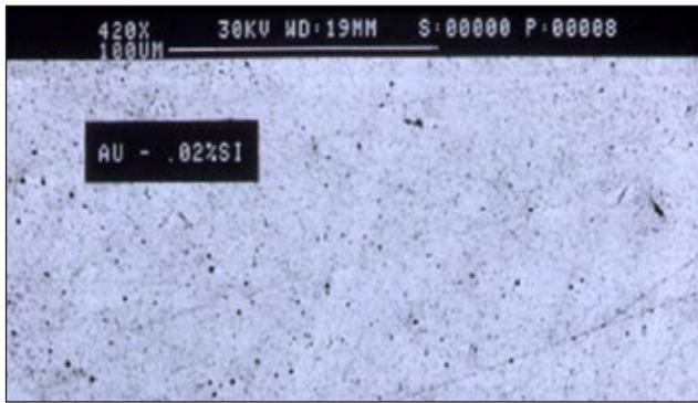
Figure 7 SEM micrograph of silicon particles dispersed in gold matrix. Average concentration of silicon measured at 200 mg/kg (424 x magnification)
