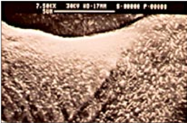
Figure 3 SEM micrograph of the surface of a grain exposed after fracture occurred in a 14K alloy. Light areas represent lead precipitate (7,500 x magnification)
