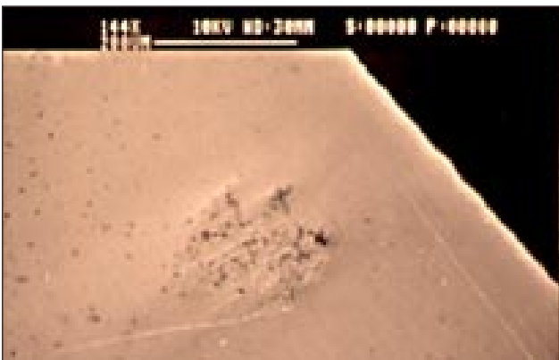
Figure 4 SEM micrograph of the surface of a 10K casting ring showing a hard spot caused by iron and boron (144 x magnification)
