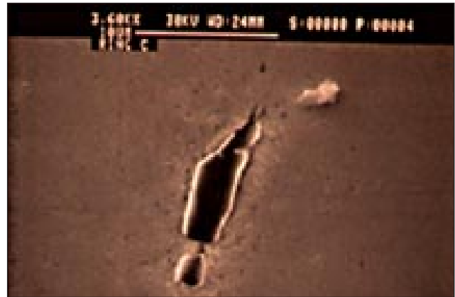
Figure 8 SEM micrograph of silicon segregation at the grain boundaries of a 10K alloy (3,360 x magnification)
