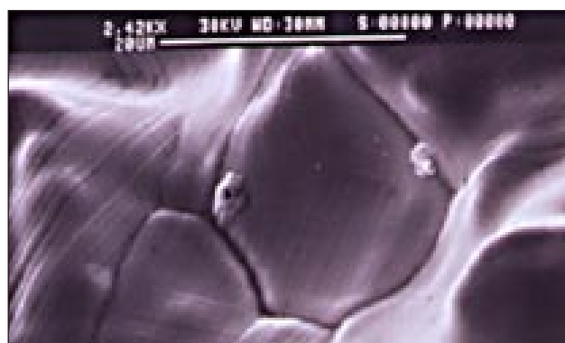
Figure 2 SEM micrograph of lead segregation at the grain boundaries of a continuously cast 14K white gold. Average lead concentration measured at 400mg/kg by atomic absorption spectroscopy (2,420 x magnification)
