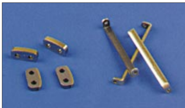
Figure 4 Two-colour gold - steel specimens fabricated from explosion welded bands and bars, respectively.
