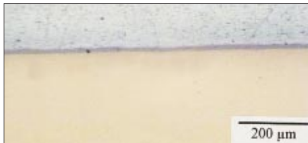
Figure 7 Micrograph of explosion welded gold-aluminum, showing the Al_2Au transition layer.
