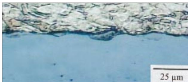
Figure 5 Micrograph displaying the flat interface of explosion welded gold-titanium.
