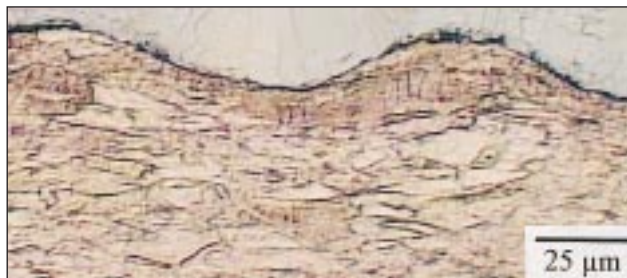
Figure 2 Micrograph showing the regular wavy yellow gold - white gold interface.
