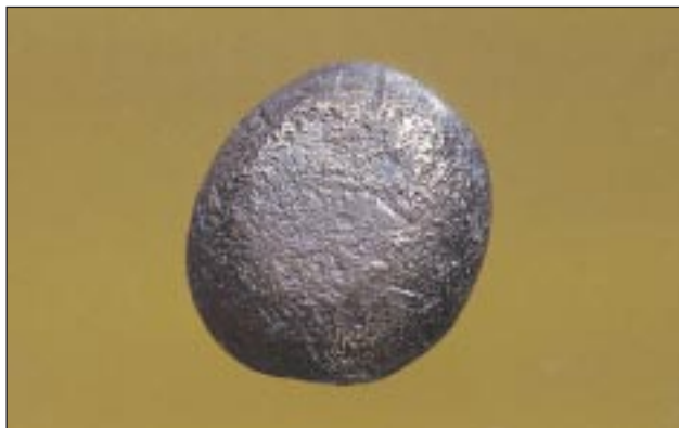
Figure 2 E1294, flan or blank prior to striking, magnification 3.5
