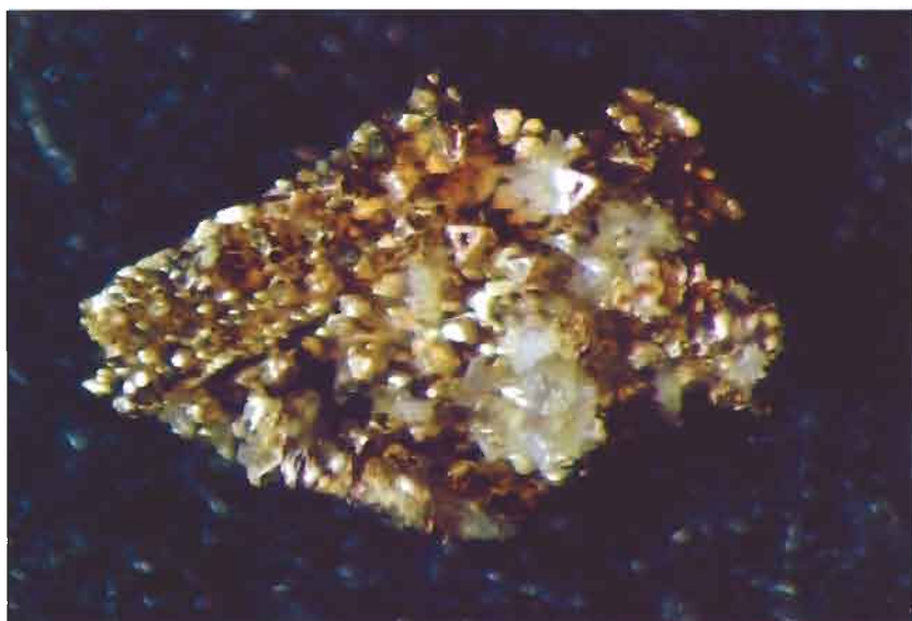
Crystalline gold recovered from alluvial workings. 'Or natif, pailleté avec fer, titane et sable du Rhin'. Brilliant sharp octahedral crystals of gold, a few of which show pseudohexagonal habit, are intimately intergrown with tiny quartz crystals less than 0.1 mm in diameter (Photo by DL)
