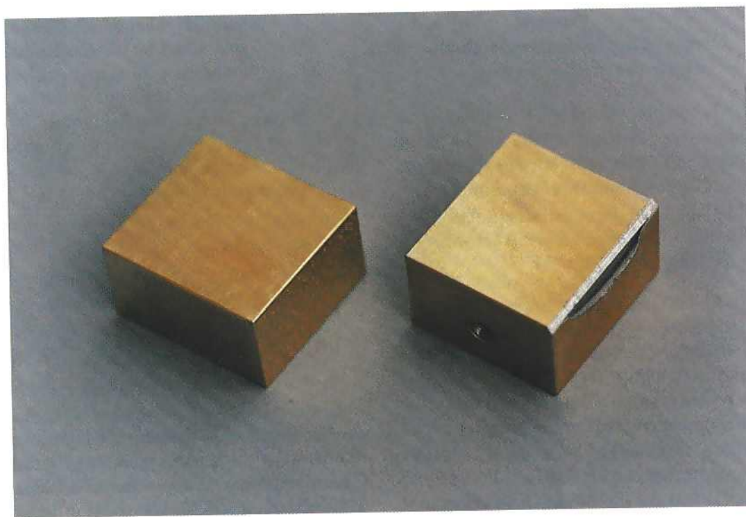
Figures 4 & 5: 6061 aluminium alloy samples after gold plating left: gold plating after a thorough pre-cleaning right: gold plating after improper pretreatment
