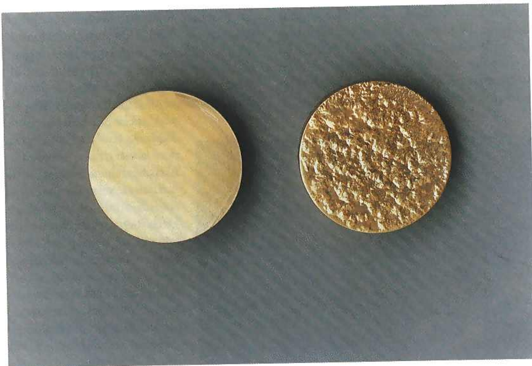
Figures 4 & 5: 6061 aluminium alloy samples after gold plating left: gold plating after a thorough pre-cleaning right: gold plating after improper pretreatment
