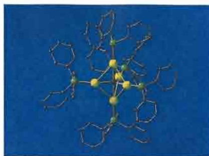
Fig. 17 Molecular structure of the monocation \{C[AuP(C_6H_5)_3]_5\}^+ in the crystal of the tetrafluoroborate salt [95]
