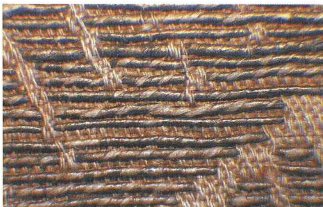
Fig 7a Scanning electron micrograph of the gold thread (width of strip: 0,70 mm) [37]
