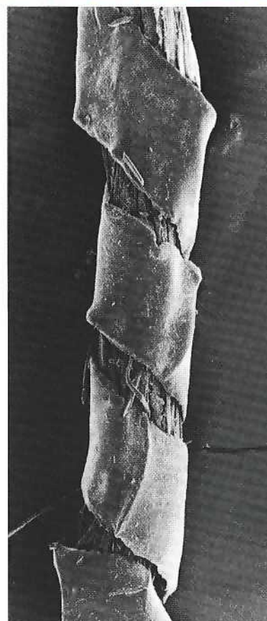
Fig. 4a Scanning electron micrograph of the gold thread (gold strip wound around a silk core; width of strip: 0.20 mm) [37]
