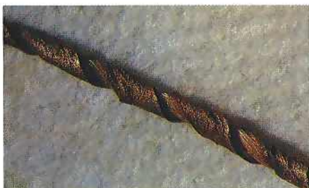
Fig. 14a Membrane thread: gilt leather strip wound around a silk core. (strip width: 0.40 mm)
