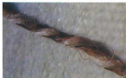
Fig. 15a Membrane thread: silver gilt animal gut strip wound around a linen core. (strip width: 0.25 mm)
