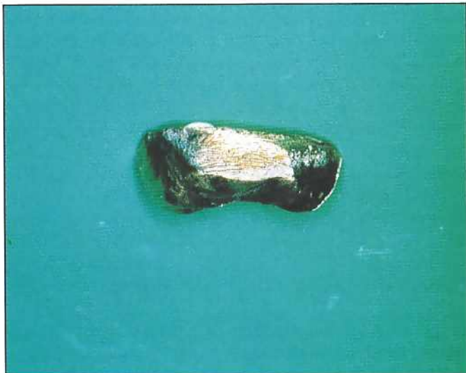
Fig. 7 Part of a crown made from a medium-gold alloy (to BS6042:1981) after being removed from a patient's mouth because of severe tarnishing. Analysis showed the base metal content of this crown to be 23.2%, probably due to contamination of the alloy during casting.
