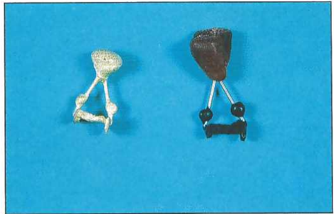
Fig. 3 A Type II dental gold inlay and a copy of the sprued wax pattern used to produce it. The patterns was invested in gypsum-bonded silica. Then this had set, the metal sprues were removed prior to heating the mould to burn out the wax and expand the mould.
