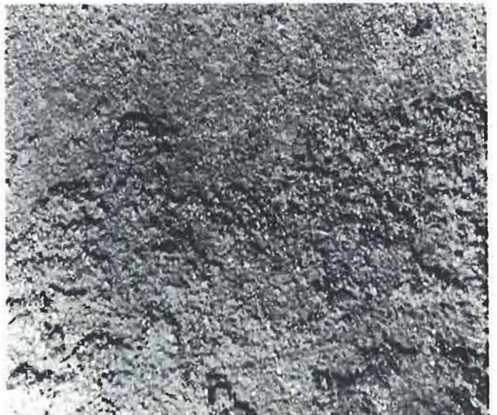
Fig. 7 Rough surface of an 18 carat gold casting formed under too high a pressure.
