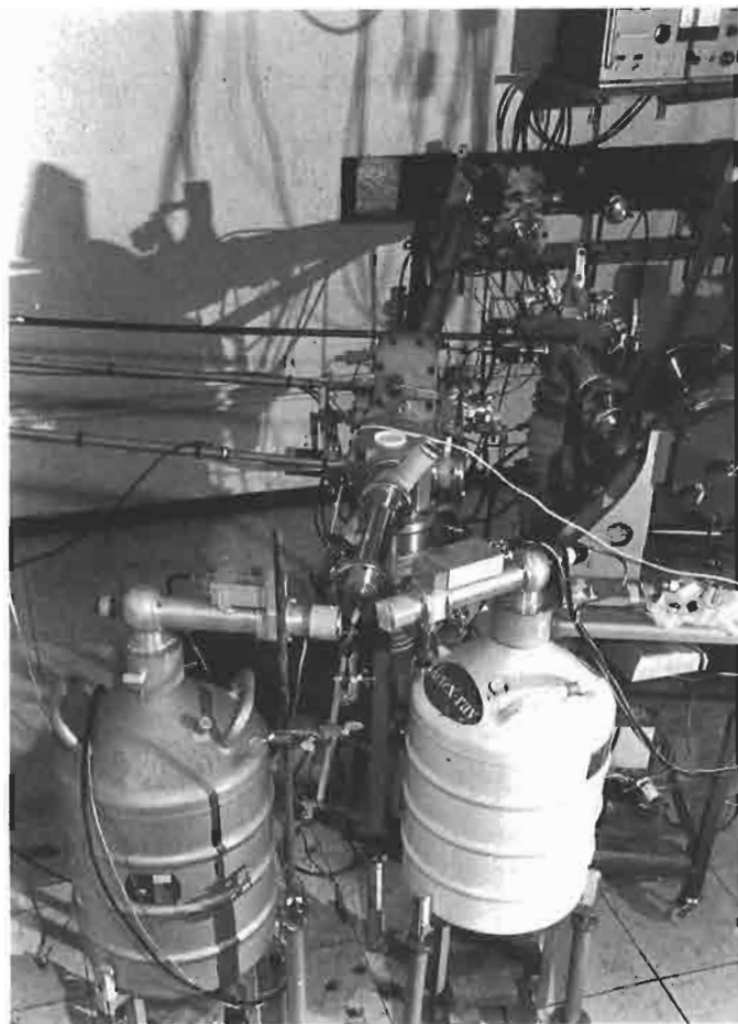
Fig. 3 A view of the PIXE apparatus showing bombardment at atmospheric pressure of an artifact, a cross, with protons extracted from the accelerator and collection of the resulting X-rays in a Si(Li) detector
