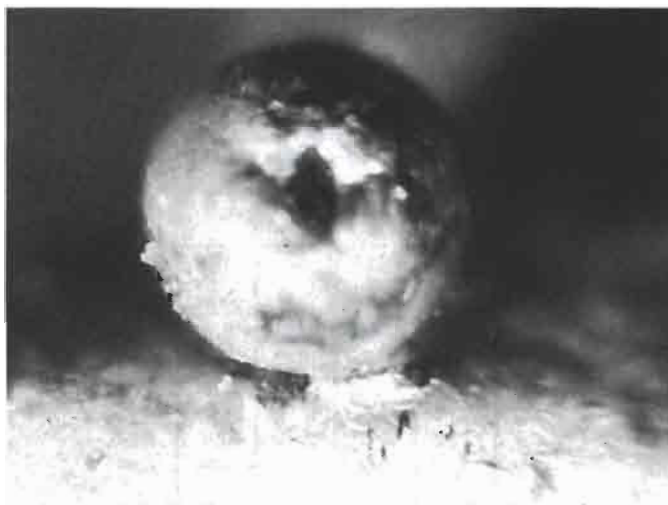
Fig. 13 Soldering by 'diffusion bonding' with greenockite. The diameter of the granule is less than 0.5 mm
