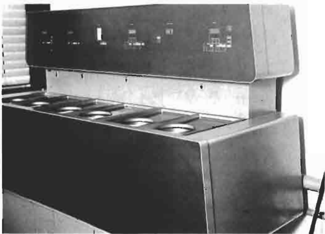
Fig. 2 M.E.M.-System electroforming apparatus as used in this study. Courtesy Oxy Metal Industries (Benelux)
