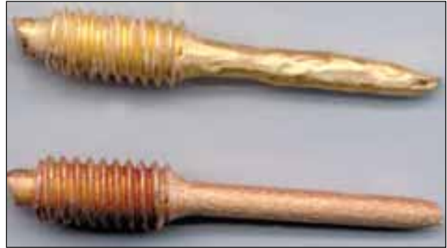
Figure 15 Fractured tensile specimens of silicon-deoxidized (top) and grain-refined (bottom) alloys showing gross, orange-peel effect on silicon-deoxidized alloy due to large grains
