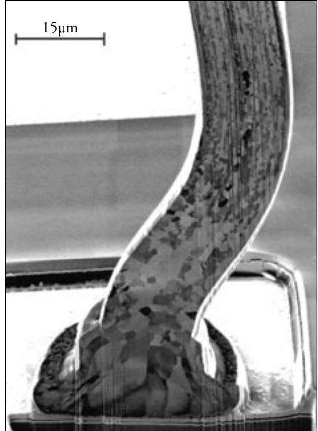
Figure 7 Photograph of a bonded low alloyed gold wire showing ball bond with deformed ball and heat affected zone
