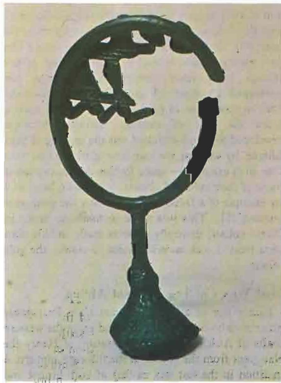
This unsuccessful casting of a similar ornament, also made in tumbaga in the Sinú region, still has its sprue in position and clearly shows the method of casting. In preparing the mould the pre-Columbian Indians mixed clay with coarsely ground charcoal, giving a porosity for the escape of air and gases so that there was no need for risers
