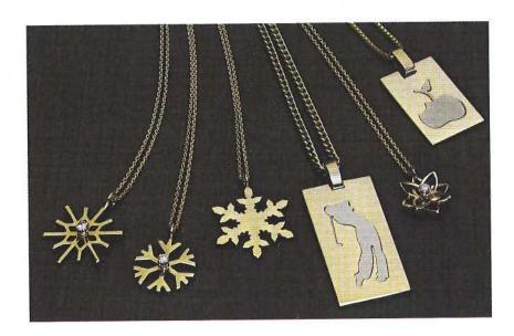
The gold pendants shown here have all been made by electrodischarge machining at Diamond Design Ltd. The 'snowflake' designs illustrate the ability of the technique to produce intricate shapes. The 'golfer' and 'apple' pendants illustrate the accuracy of EDM. They were made by machining the yellow gold cut-out profiles and the white gold residual profiles in separate operations and by sleeving them together
