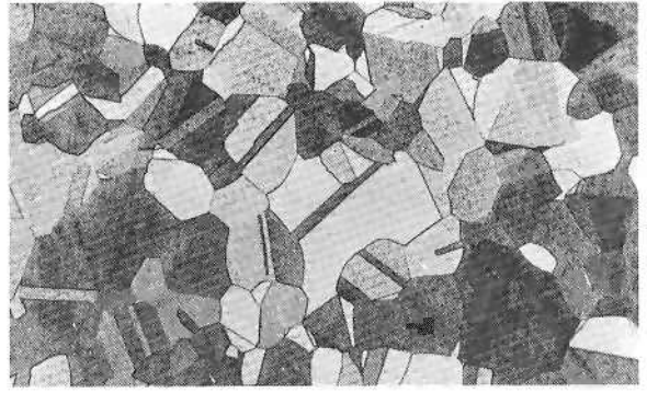
Fig. 2 18 carat yellow gold + 0.5% Fe, annealed 1 hour, 700°C, × 100
