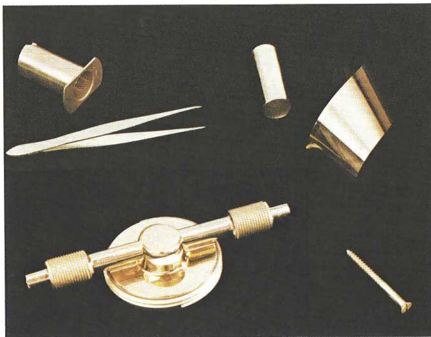
Fig. 3 The versatility of ion plating is illustrated by examples of components of various shapes and materials which were gold coated by the process. Clockwise, the objects in this photograph are: a piece of stainless steel tubing, a piece of polyimide plastic foil, a steel screw, a valve moulding of Polyethersulphone (an icl plastic), a pair of stainless steel tweezers and a part of a polypropylene syringe. The gold coatings on all these objects are in the range 2000 to 5000 Å thick
