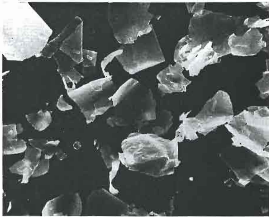
Fig. 1 This powder was made by breaking down gold leaf. The random shape of the flake-like particles is obvious, although there are also a few crystals present \times 625
