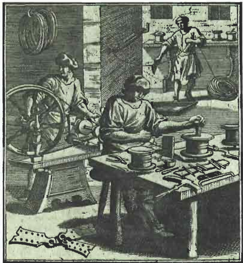
Fig. 3 An engraving showing the drawing of gold and silver wire at the end of the seventeenth century, from the Abbildung der gemein nützlichen Hauptstände by Christoph Weigel, published in Regensburg in 1698
