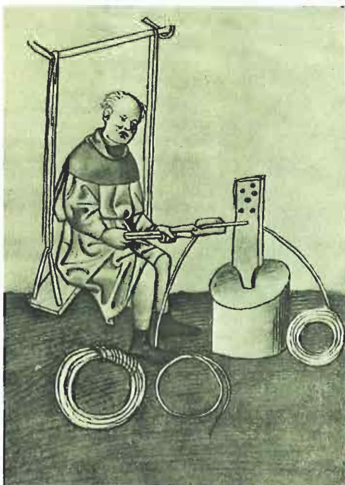
Fig. 1 Probably the first illustration of wire-drawing through a draw-plate, this picture from a manuscript of A.D. 1389 the Hausbuch compiled in Germany by the Mendel Brothers, shows a monk sitting on a swinging seat so that he can push backwards with his legs against the anvil holding the draw plate, the tongs holding the wire being fastened to his belt
