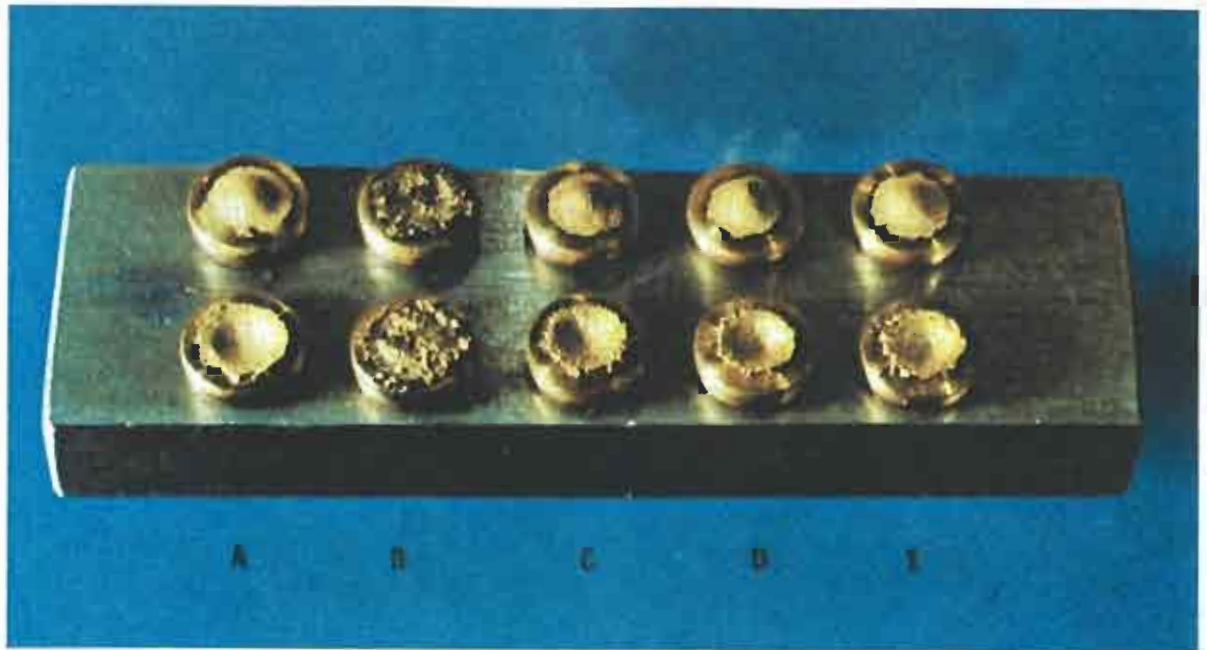
Fig. 2 Arc erosion of gold and dispersion-strengthened gold alloys, after 7000 operations, with an 80-ampere make-arc. Upper Contact: Cathode, Lower Contact: Anode
