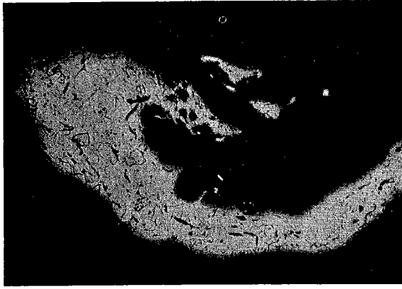
A section from the suit of armour made for Prince Charles. The only constituents visible are grains of ferrite and slag inclusions. The gold layer is unfortunately too thin to be visible ×100
