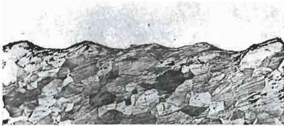
Fig. 5 Photomicrograph of gold clad nickel. \times 100
