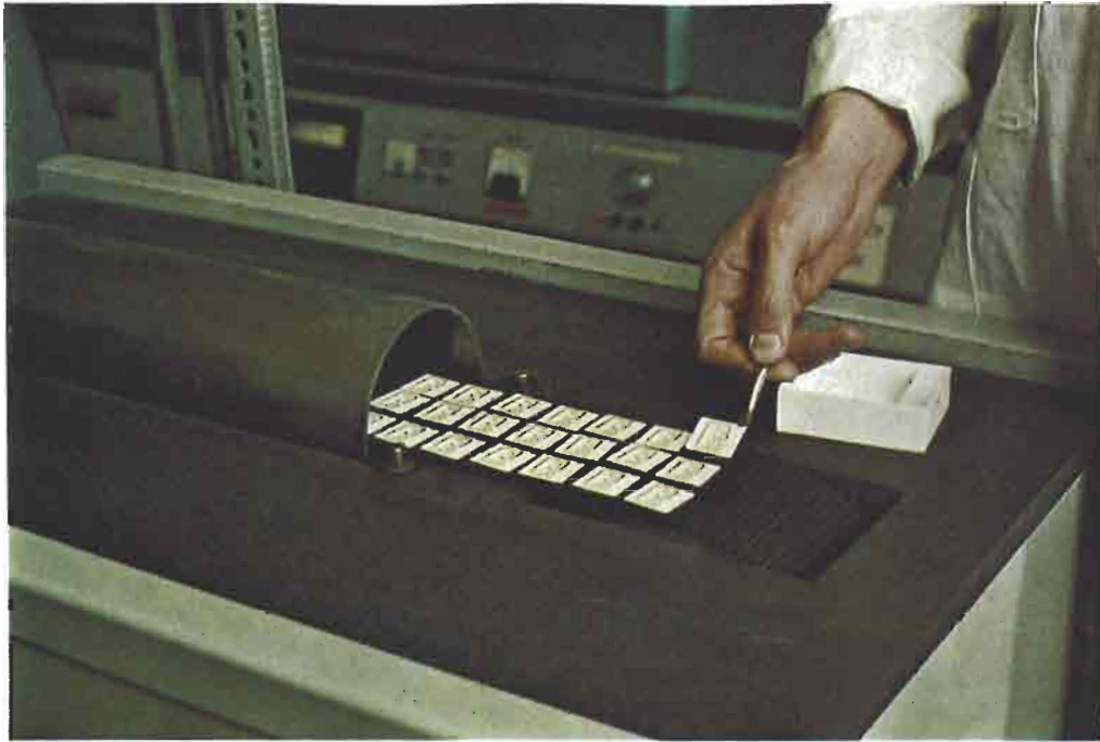
Thick-film gold conductors fired on to ceramic substrates emerging from a continuous belt furnace. The firing operation sinters the gold particles and promotes bonding either reactively between oxides in the film and the alumina of the ceramic or by glass bonding. Firing is usually in air, and peak temperatures do not normally exceed 1000°C
