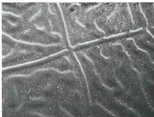
Fig. 4 Scanning electron micrographs of the surface of a gold-cobalt deposit after annealing for 1 hour at 400°C Fig. 4a (top) ×40, Fig. 4b (bottom) ×4000
