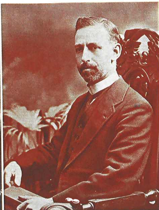
The same sulphide-toned print which has since been gold-toned. The brown tones have changed quite dramatically into a brilliant red colour, the image now consisting of a double sulphide of gold and silver
