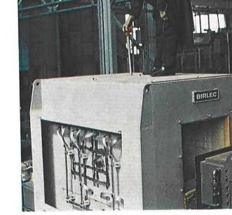
Gold-palladium alloy thermal fuses are fitted to high temperature furnaces, both of the general purpose batch type and the continuous belt conveyor type. Here a fitter is inserting the fuse through the roof of a hump-back mesh belt conveyor furnace being constructed by Birlec Limited for use in the heat treatment of stainless steel components in a special controlled atmosphere
