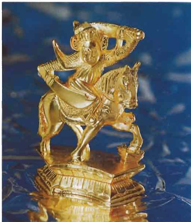
Chesspiece with a wall thickness of about 375 micrometres made from a solid wax model
