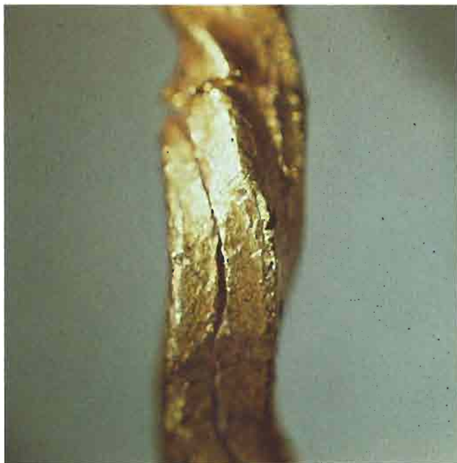
Fig. 6 Detail of cracks in a twisted torc made from rod in square cross-section (Necklace from Jaligny-sur-Besbre, Allier, France). Middle Bronze Age, 1500-1200 B.C.
