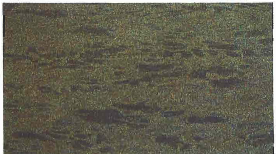
Fig. 4 Microstructure of shakudo containing 5% gold × 60
