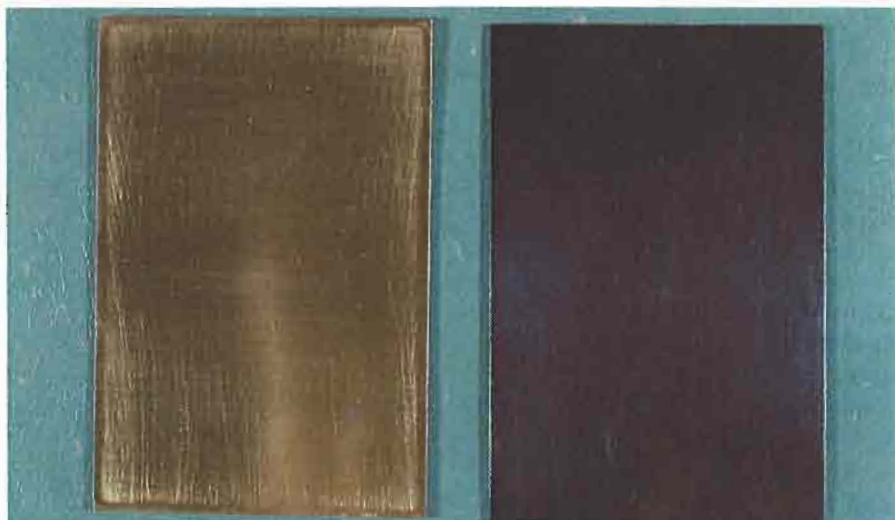
Fig. 8(a) Surface colours of shakudo containing 5% Au. Full size Left: Surface colour of shakudo before treatment Right: Black colour of shakudo after treatment
