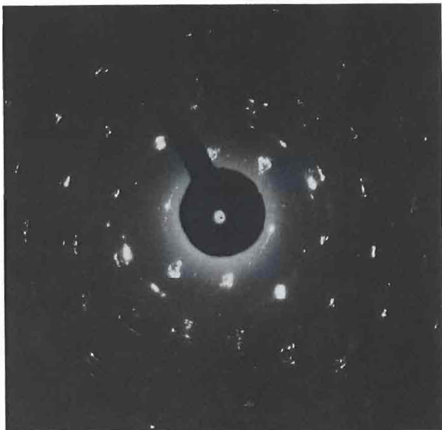
Fig. 10(b) Diffraction pattern of sample shown in the electron micrograph in Fig. 10(a)
