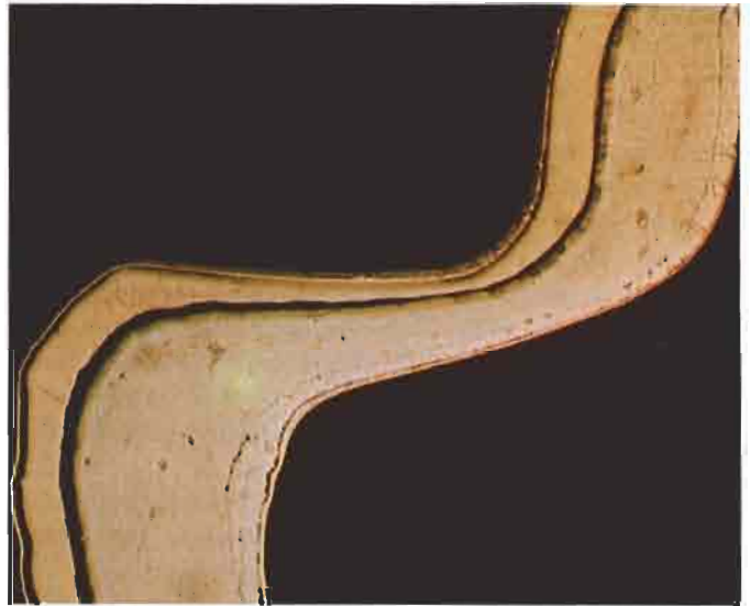
Fig. 2 Photomicrograph of a rolled gold watch case. The thickness of the gold layer (the thinner of the two sections) has been reduced by almost 50 per cent in the areas of maximum stretching and deformation
