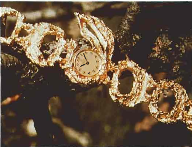
Fig. 6 Heavy gold electroplate was applied to natural seashells which were subsequently dissolved by acid and the 'hole' soldered over leaving an electroformed hard pure gold product
