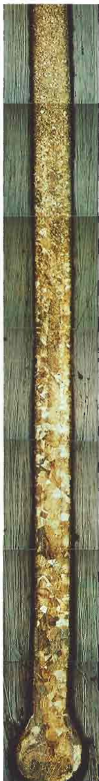
Fig. 10 Grain growth in the portion of a gold bonding wire heated during ball formation
